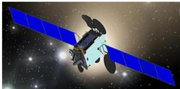
Es'hail-2 will carry two AMSAT-DL-designed Phase 4 Amateur Radio transponders operating in the 2.4 GHz and 10.450 GHz bands. A 250 kHz
