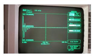
It is a screen shot of a transmitter 'fingerprint'. I had repaired an Icom IC3AT HT with a new power amp transistor. I wanted to see if it had
